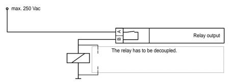
Figure 4-12: Controller - SPM-D2-11/LSXR - three-position controller
