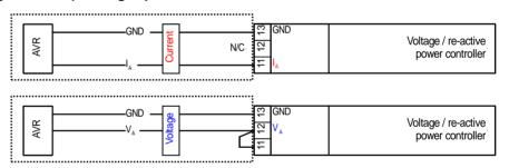
Figure 4-14: Controller - SPM-D2-11/LSXR - Analog controller output - Voltage/power factor
