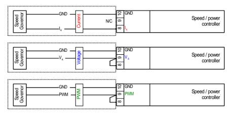
Figure 4-13: Controller - SPM-D2-11/LSXR - Analog controller output - Speed/frequency/real power
