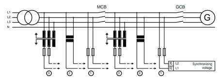
Figure 4-5: Measuring inputs - Synchronization voltage
