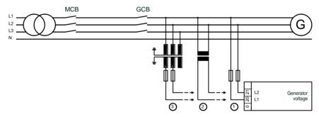
Figure 4-4: Measuring inputs - Generator
