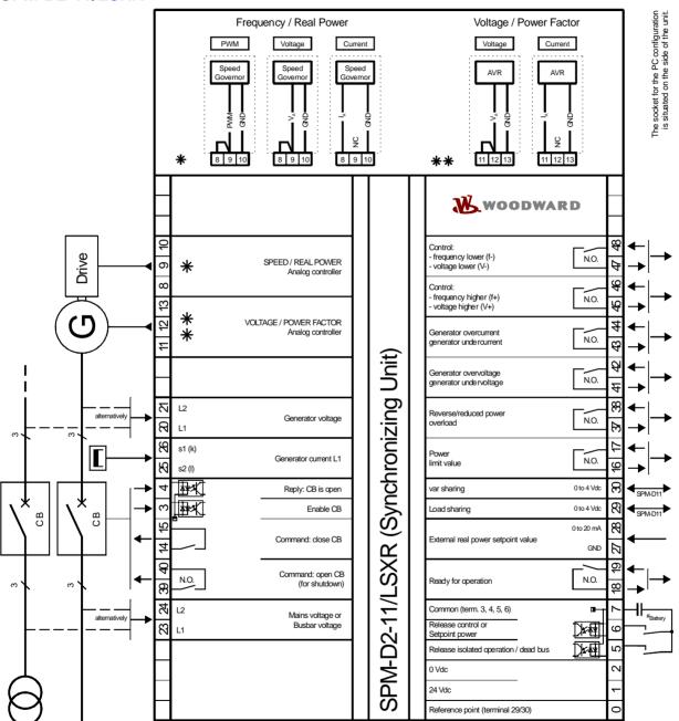
Figure 4-1: Wiring diagram SPM-D2-11/LSXR
