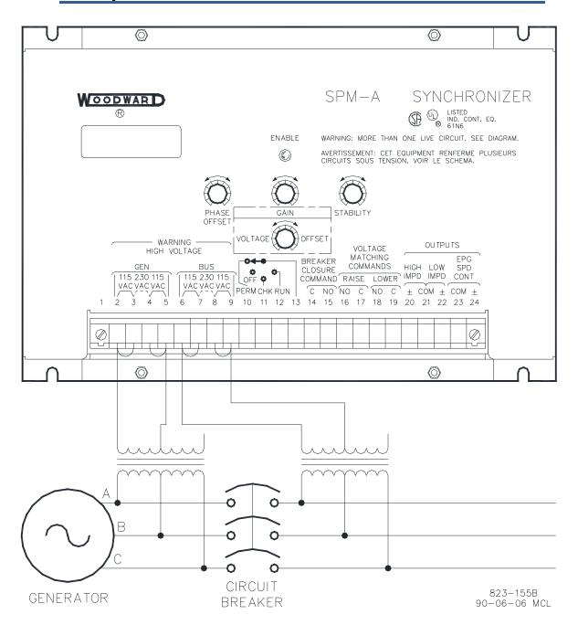
Figure 2-1. Typical SPM-A Synchronizer Wiring
