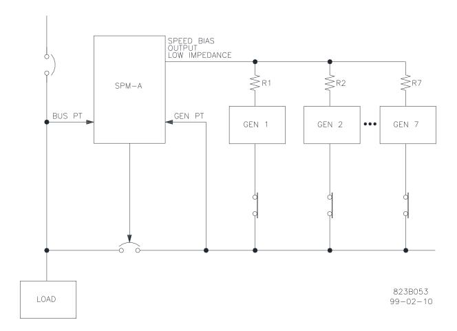
Figure 2-2. Synchronizing Bus to Bus
