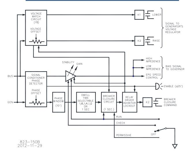
Figure 1-3. Functional Block Diagram
