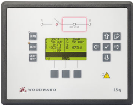
Fig. 5: Display LS-522 configured as LS-521
