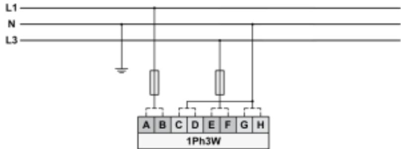
Fig. 35: Measuring inputs - 1Ph 3W
