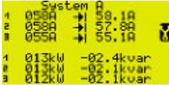
Fig. 101: Slave pointer system A screen (example)
