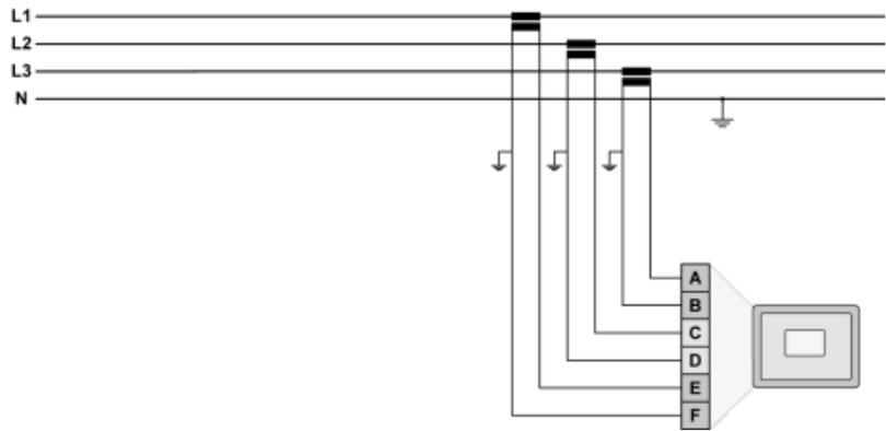
Fig. 38: Current measuring - system A - wiring
