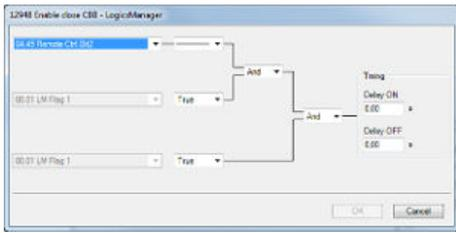
Fig. 142: LogicsManager configuration "Enable close CBB"
