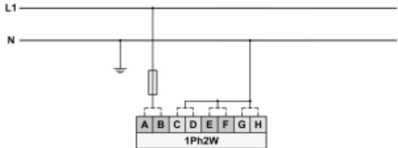
Fig. 36: Measuring inputs - 1Ph 2W (phase neutral)
