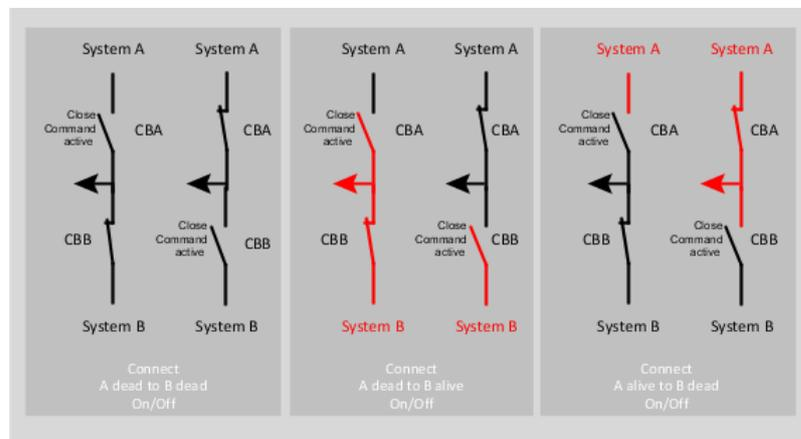
*Fig. 66: Dead busbar: System A/B closure*
