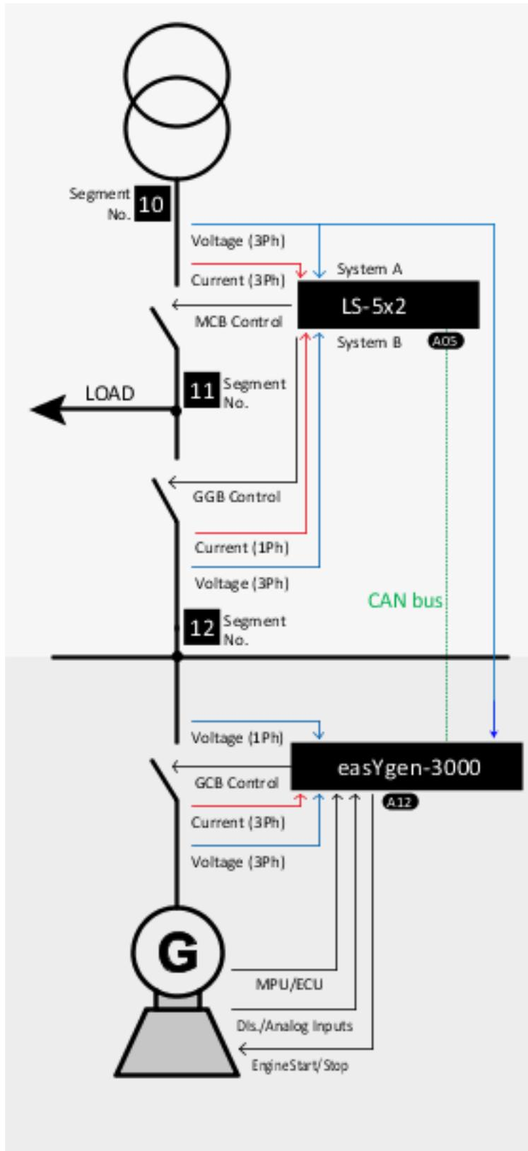
Fig. 146: One easYgen-3500XT with one LS-5x2 (example)
