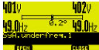
Fig. 128: LS-5x2 v2 Synchroscope in operating mode MANUAL (example)
