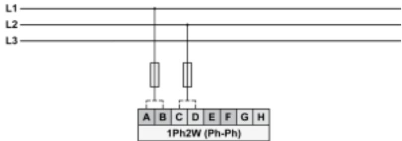
Fig. 37: Measuring inputs - 1Ph 2W (phase-phase)
