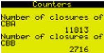
Fig. 121: CBA and CBB close counters screen (example)
