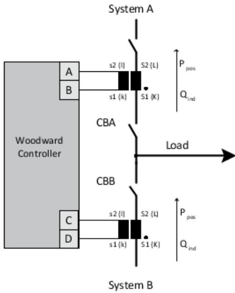
Fig. 43: Power measuring - wiring
