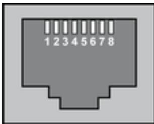
Fig. 54: Service port connector (RJ-45)
