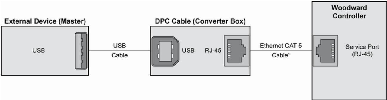
Fig. 55: DPC-USB wiring - schematic
