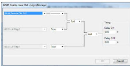
Fig. 141: LogicsManager configuration "Enable close CBA"
