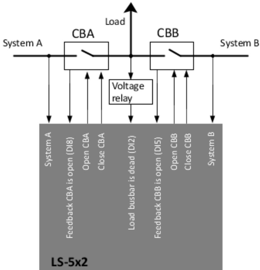
Fig. 148: Example: The voltage relay informs by DI 2 about the load busbar condition.
