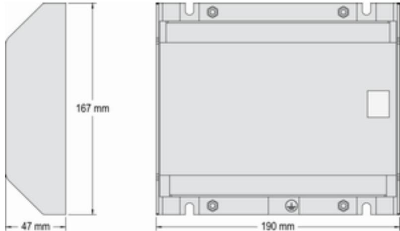
Fig. 8: Sheet metal housing - dimensions
