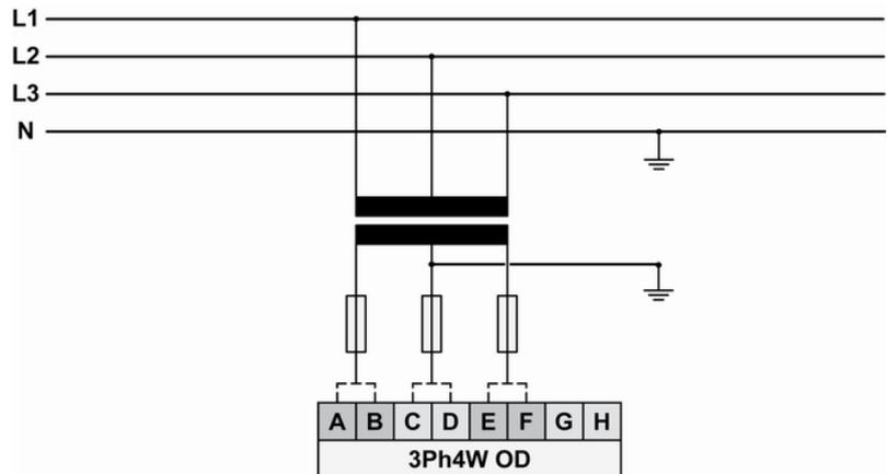
Fig. 26: Measuring inputs - 3Ph 4W OD
