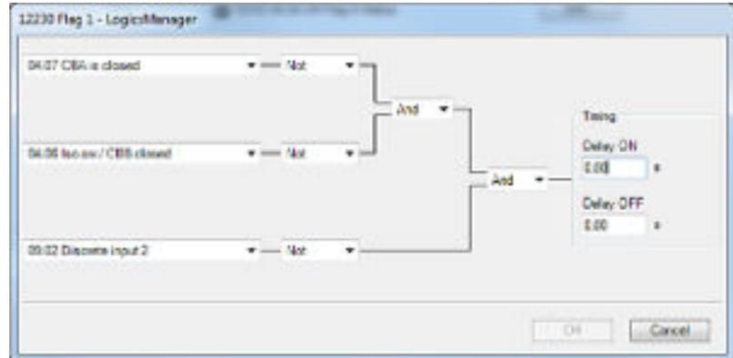
Fig. 150: Toolkit: Configuration of the failure flag (LogicsManager Flag 1) (example)
