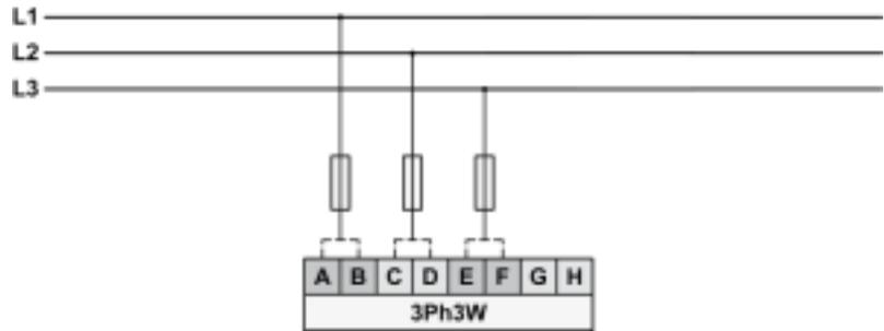
Fig. 34: Measuring inputs - 3Ph 3W
