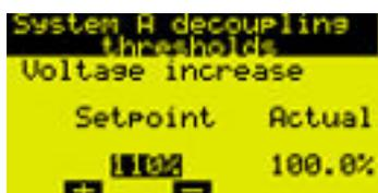
Fig. 117: Decoupling voltage increase (example)
