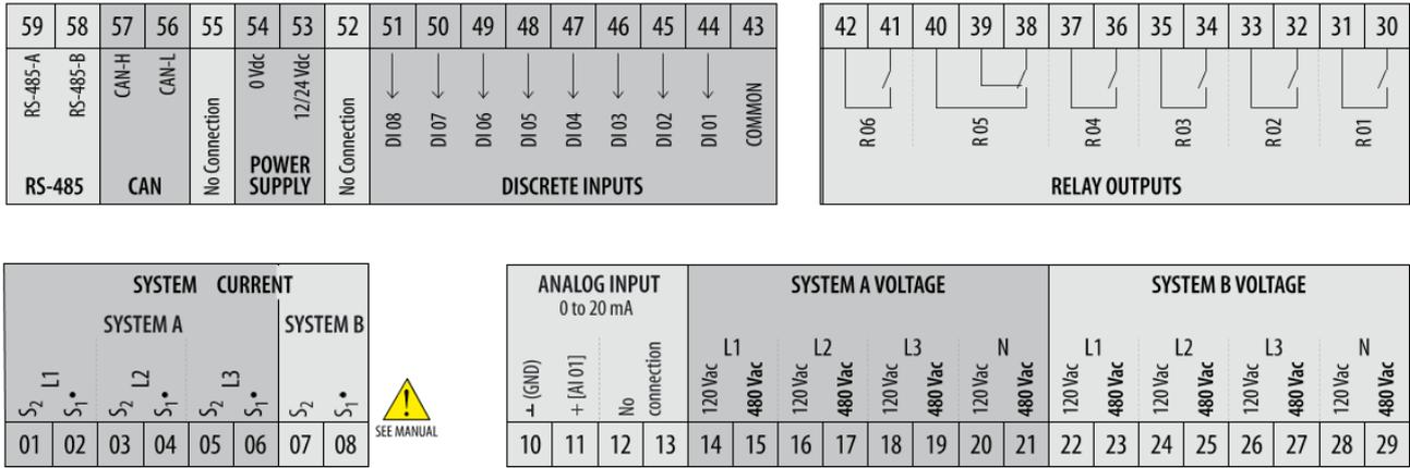
Fig. 20: Label/print LS-5x2 v2 series wiring
