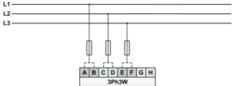
Fig. 28: Measuring inputs - 3Ph 3W
