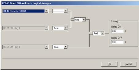
Fig. 143: LogicsManager configuration 'Open CBA unload'
