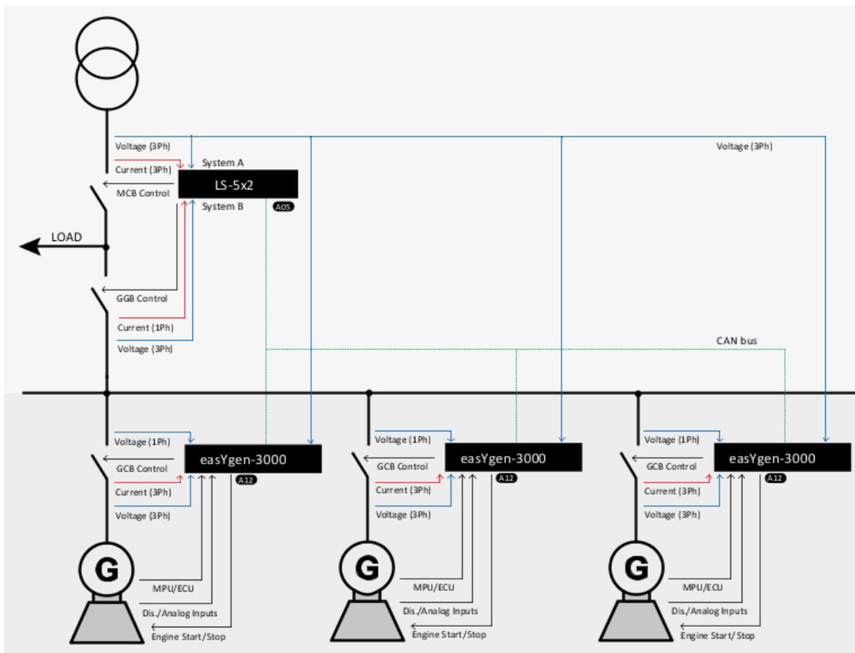
Fig. 147: Multiple easYgen-3500XT with one LS-5x2 (example)
