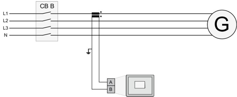
Fig. 41: Current measuring - System B - wiring (example)
