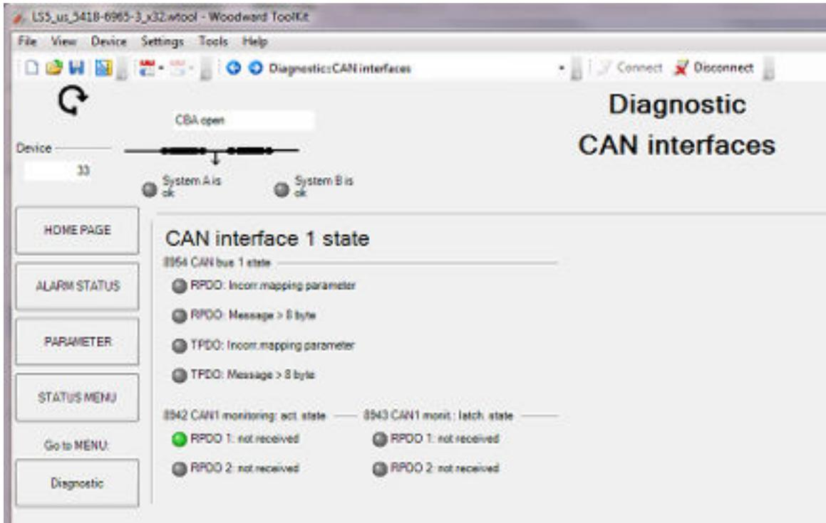
Fig. 86: CAN interface state screen (example)
