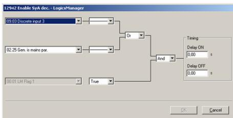
Fig. 134: LogicsManager configuration example 2
