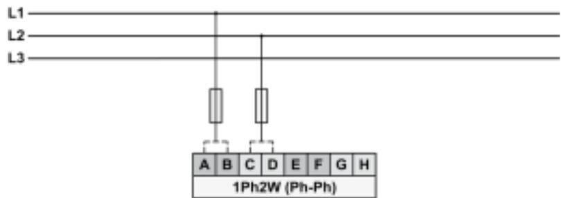
Fig. 31: Measuring inputs - 1Ph 2W (phase-phase)
