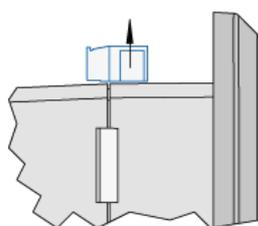
Fig. 12: Remove terminals
