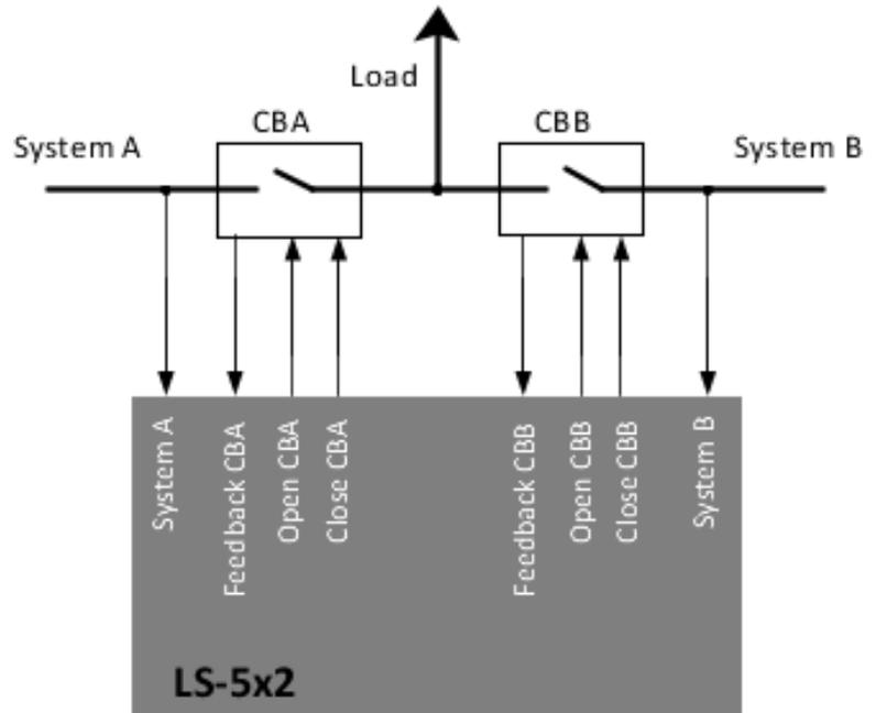
Fig. 24: LS-5x2 v2 Voltage measuring
