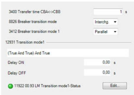
Fig. 140: Configure the breaker transition mode
