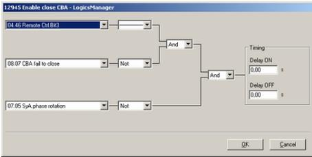
Fig. 145: LogicsManager configuration 'Enable close CBA.'
