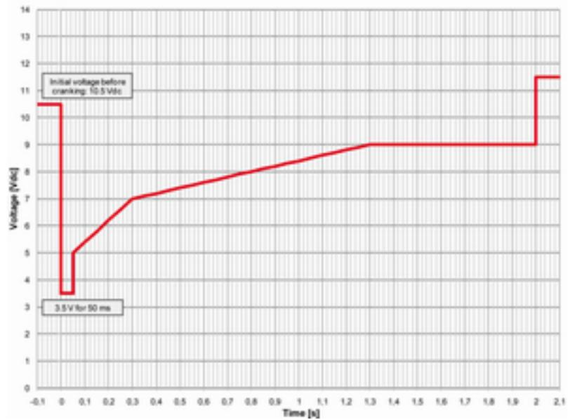
Fig. 23: Power supply - crank waveform
