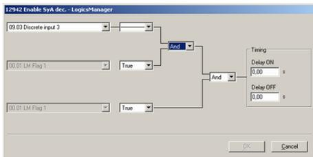
Fig. 133: LogicsManager configuration example 1
