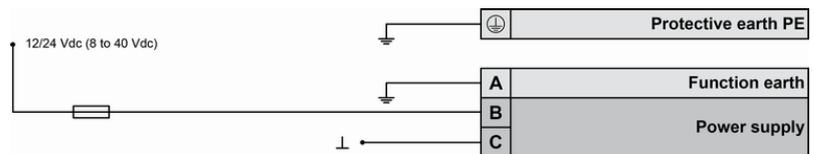
Fig. 22: Power supply - wiring
