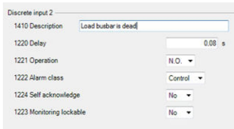
Fig. 149: Toolkit: Configuration of the discrete input 2 (example)
