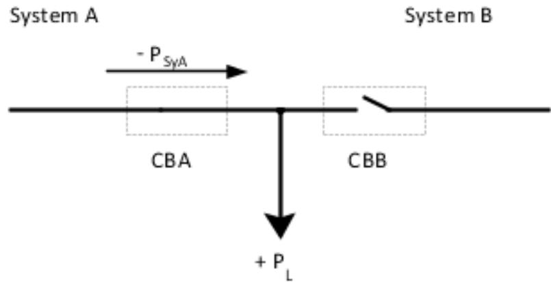
Fig. 44: LS-5x2 v2 Power measuring CBA closed
