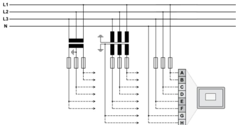
Fig. 25: Voltage measuring - system A - wiring
