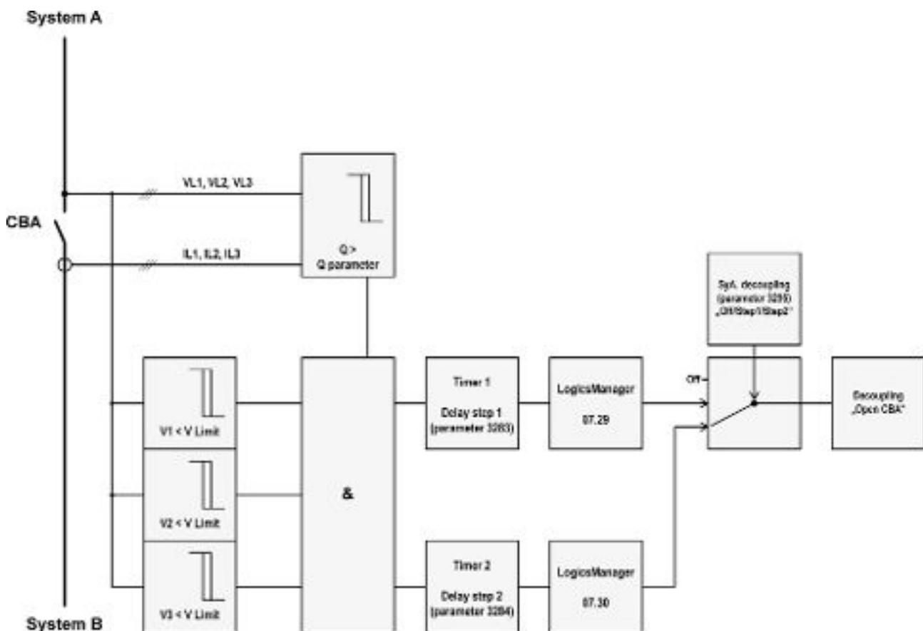
Fig. 63: QV monitoring - schematic
