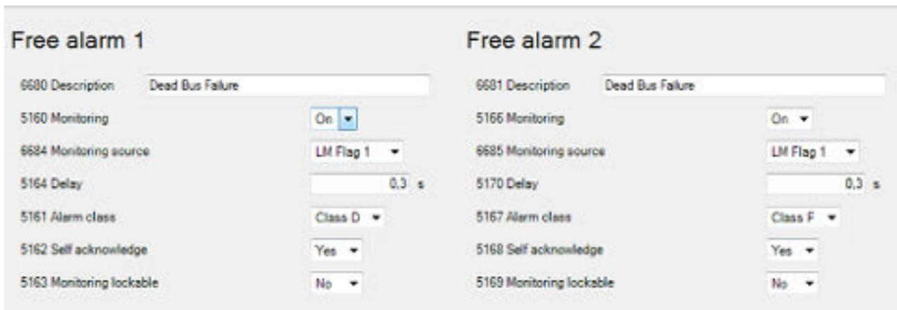
Fig. 151: Toolkit: Configuration of two alarms to block both breakers (example)
