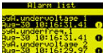
Fig. 99: Alarm List screen (example)
