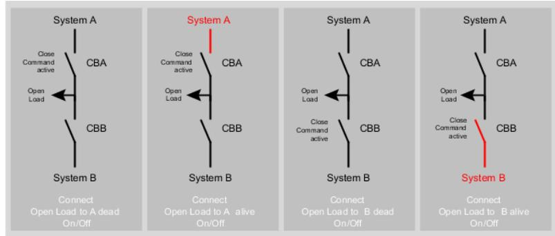
Fig. 65: Dead busbar: Open load segment closure
