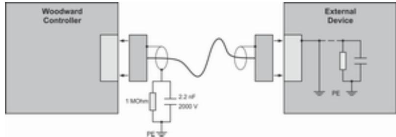
Fig. 58: Bus shielding (external RC element)
