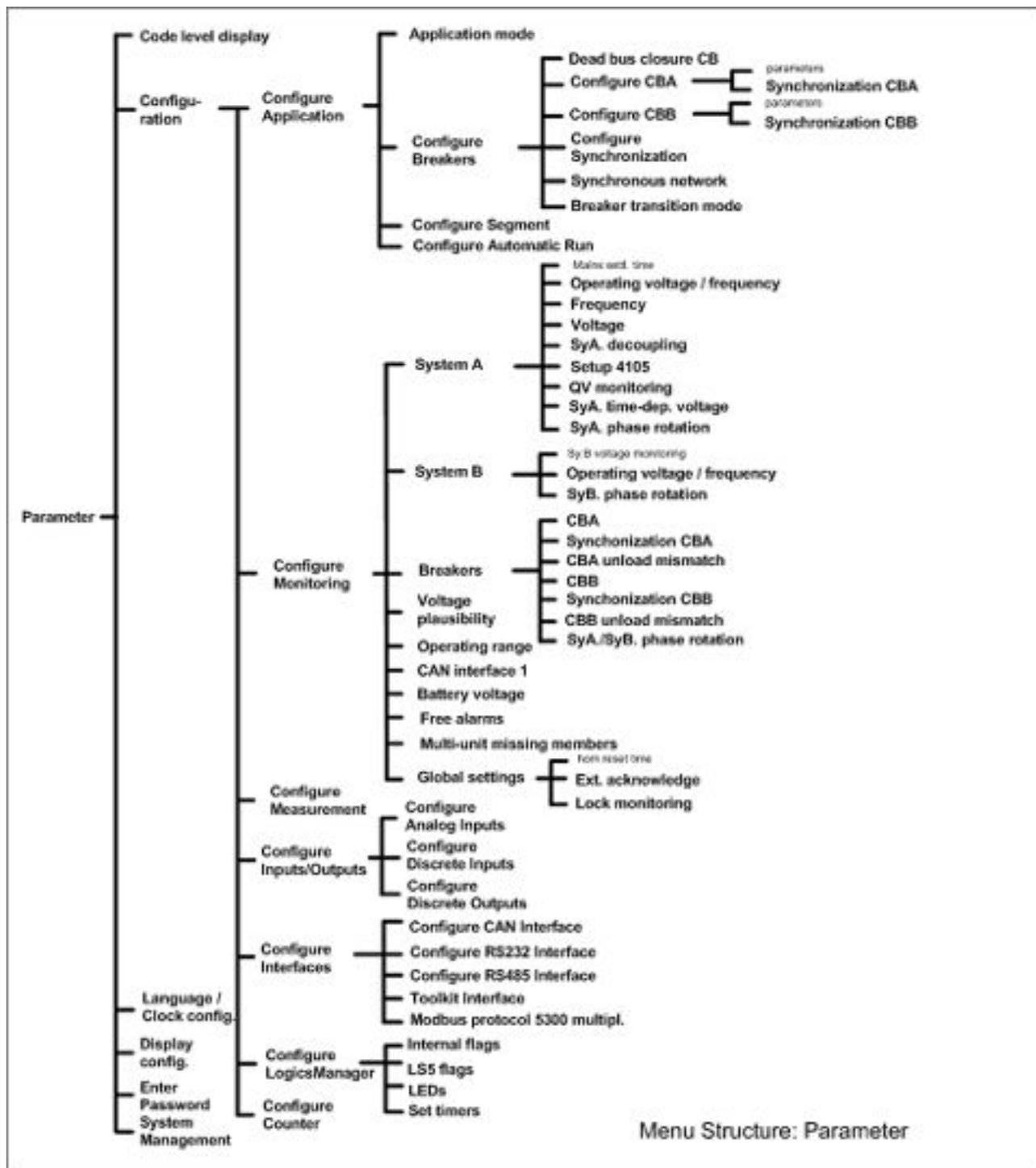
Fig. 91: Menu structure - Parameter
