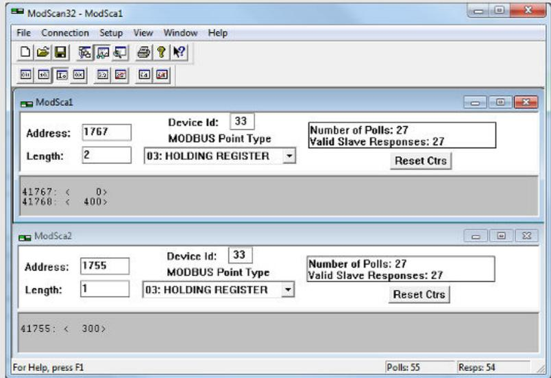
*Fig. 159: ModScan to handle 1 and 2 bytes data types*
