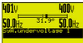
Fig. 105: Synchroscope screen (example)
