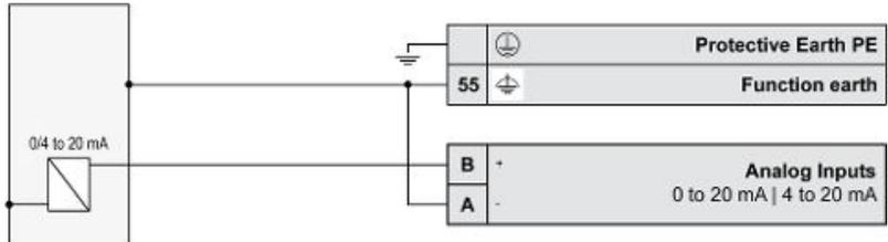
Fig. 47: Analog input - wiring single-pole sender (20 mA)
