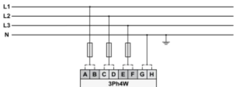
Fig. 27: Measuring inputs - 3Ph 4W
