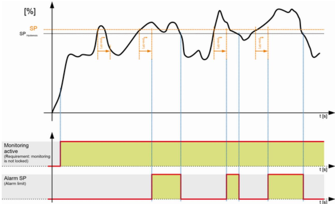
Fig. 164: One-level asymmetry monitoring
