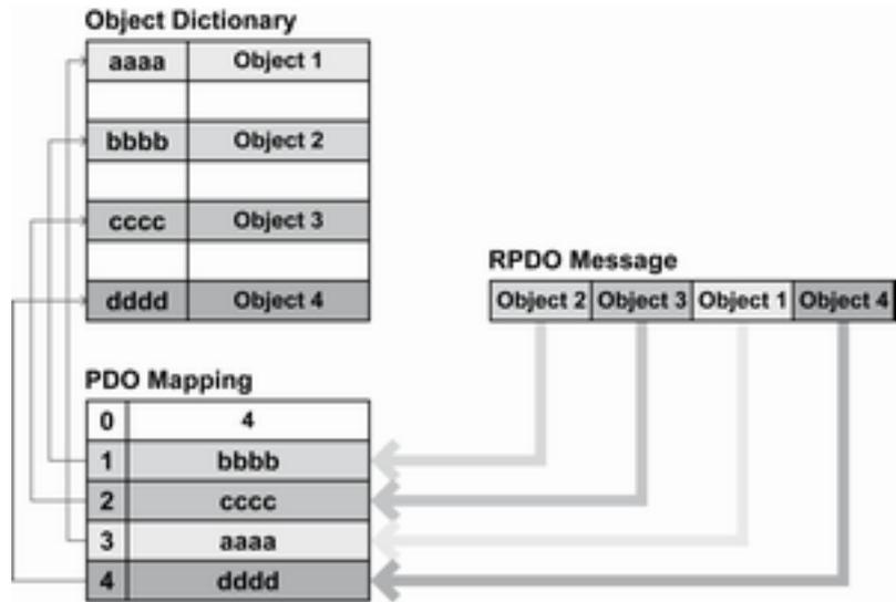
Fig. 70: RPDO mapping principle
