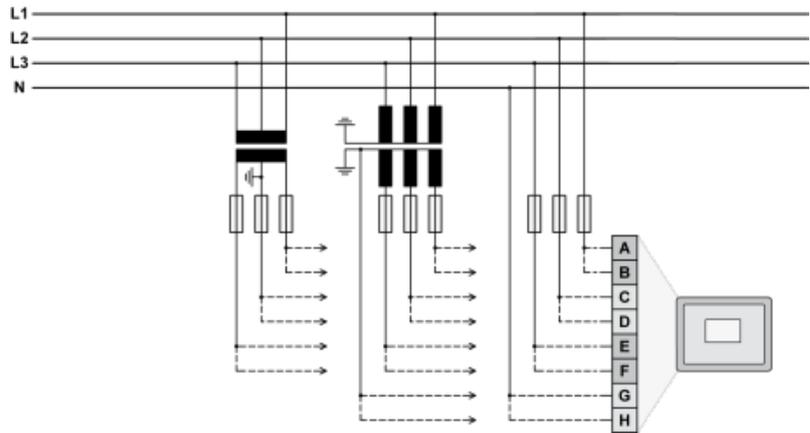
Fig. 32: Voltage measuring - system B - wiring
