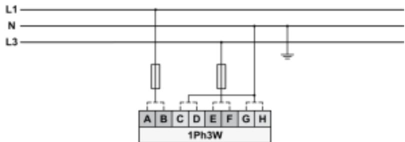
Fig. 29: Measuring inputs - 1Ph 3W
