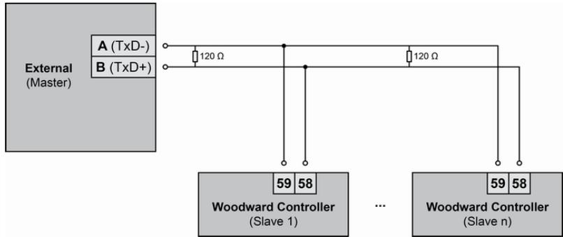
Fig. 53: RS-485 - connection for half-duplex operation
