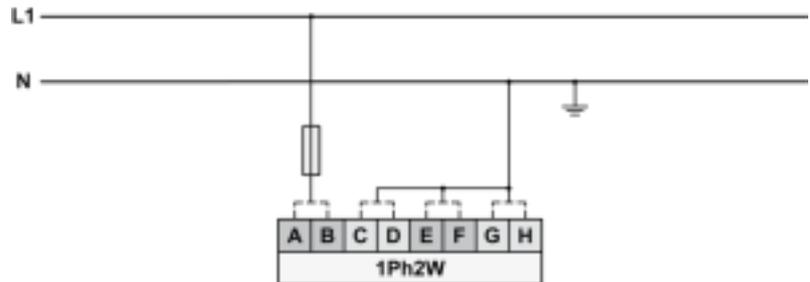
Fig. 30: Measuring inputs - 1Ph 2W (phase neutral)
