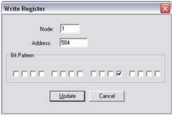
Fig. 268: Modbus - write register - external acknowledge
