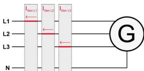
Fig. 45: Current measuring - generator, L1 L2 L3
