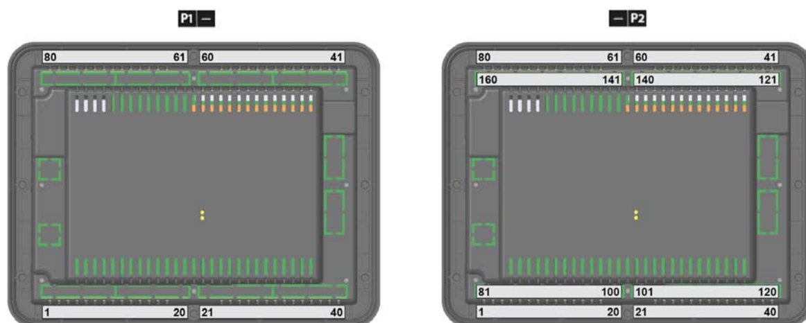
Fig. 19: easYgen-3500 plastic housing
