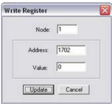
Fig. 307: Write register - resetting the default values
