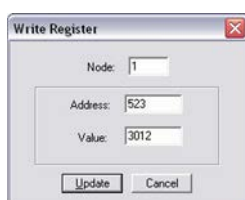
Fig. 301: Write register - acknowledge alarm message
