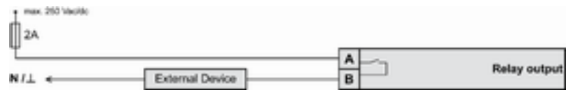
Fig. 52: Relay outputs - schematic
