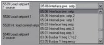
Fig. 208: Setpoint source configuration
