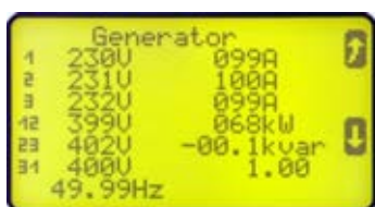
Fig. 125: Status/Monitoring screen (example)
