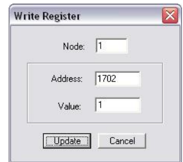
Figure 10-13: Modbus - write register - resetting the default values
