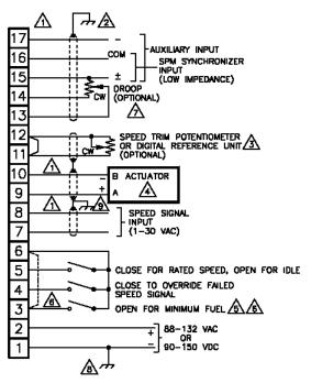
**High Voltage Version Plant Wiring Diagram**
