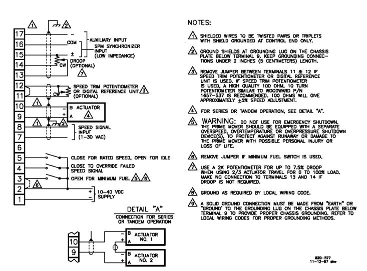
**Low Voltage Version Plant Wiring Diagram**
