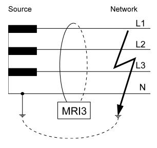
Figure 4.8: System earth fault protection
