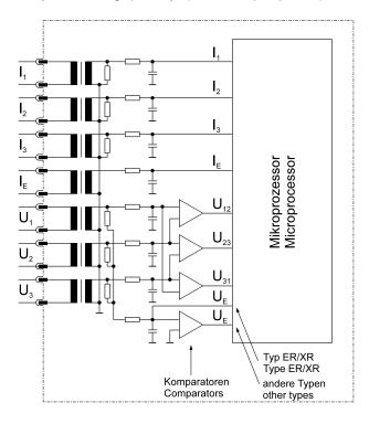
Figure 4.1: Block diagram
