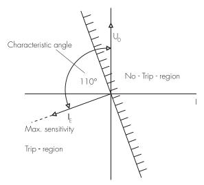
Figure 4.11: Characteristic angle in solidly earthed-systems (SOLI)
