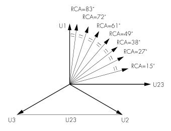
Figure 4.2: Relay characteristic angle
