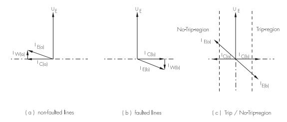
Figure 4.9: Phase position between the residual voltage and zero sequence current for faulted and non-faulted lines in case of isolated systems (sin φ)
