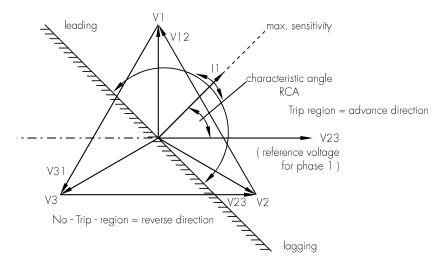
Figure 4.6: TRIP/NO-TRIP region for directional element in MRI3. In this case the foreward direction is defined as TRIP region and the backward direction as NO-TRIP region.
