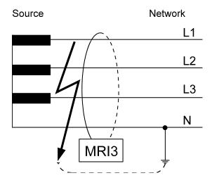
Figure 4.7: Generator stator earth fault protection
