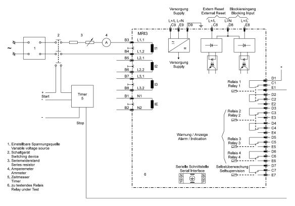
Figure 6.1: Test circuit
