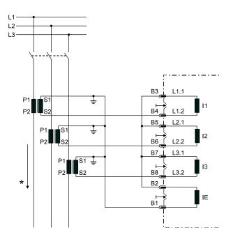
Figure 3.3: Phase current measuring and earth-current detection by means of Holmgreen-circuit.
