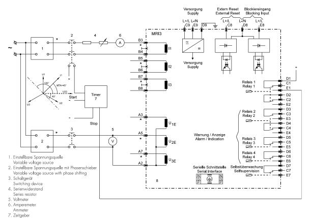
Figure 6.2: Test circuit
