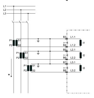
Figure 3.1: Measuring of the phase currents for over-current- and short-circuit protection (I>,I>>)
