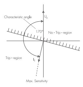
Figure 4.12: Characteristic angle in resistance-earthed systems (RESI)
