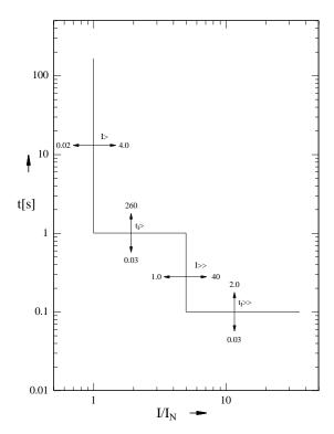
Figure 7.7: Definite time overcurrent relay
