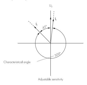
Figure 4.13: Adjustable characteristical angle of 45° to 309°
