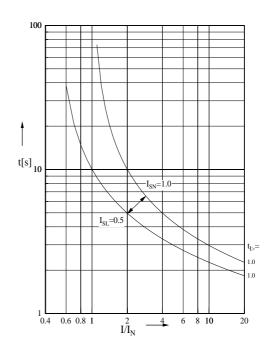
In case of failure (short-circuit of the alternator) the alternator voltage decreases. The *MRI1-IU* will recognise this and then switch over without delay to a lower pickup value IS. The value ISL can be adjusted. As a result, shorter tripping periods of the overcurrent and short-circuit step can be achieved. The adjusted tripping characteristics (normal inverse, very inverse, extremely inverse or DMT is maintained). Setting ranges see in 7.3.
