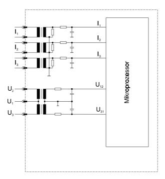
Figure 4.1: Block diagram
