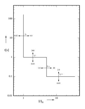
Figure 7.4 Definite time overcurrent relay
